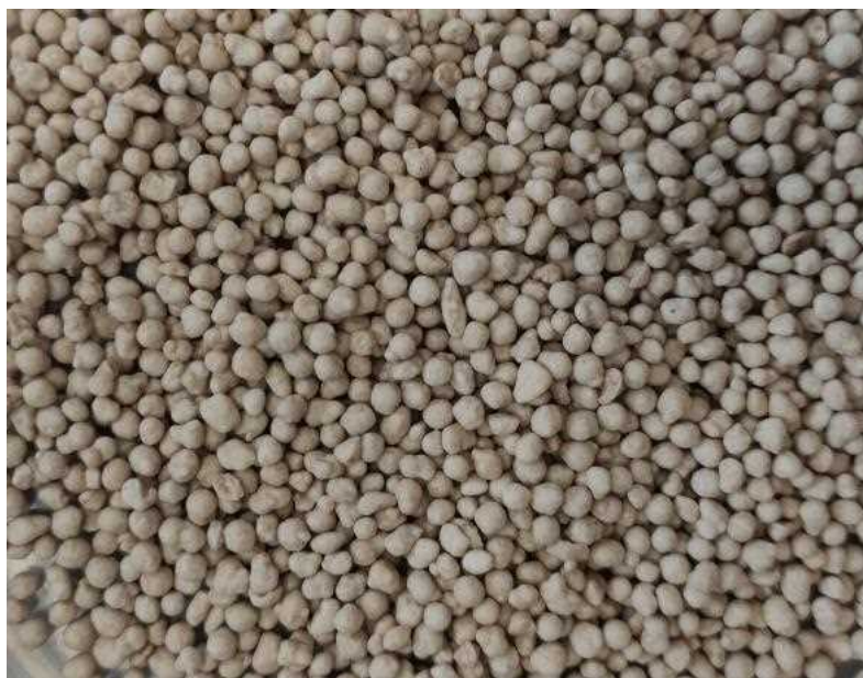
Fig. 3. NCaS fertilizer granules obtained during semi-technical tests.
