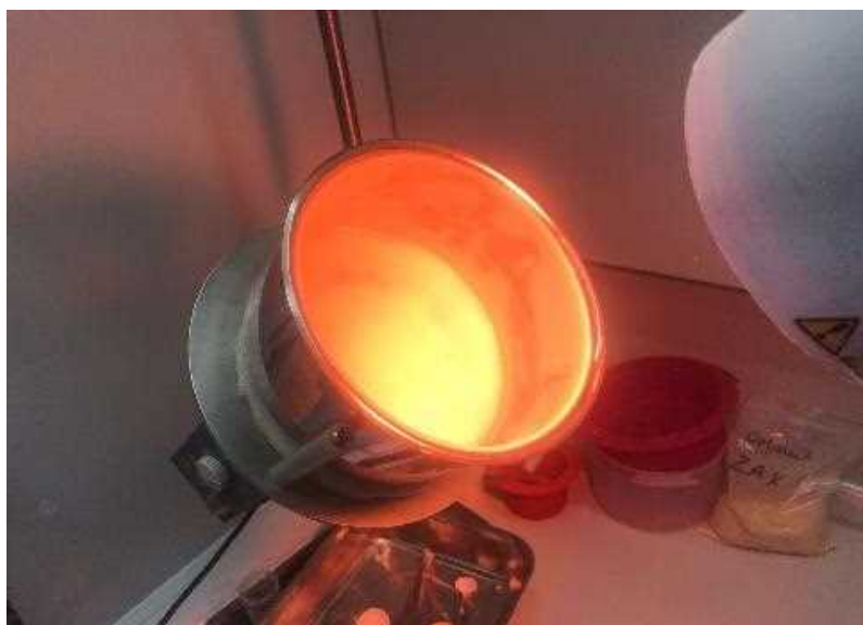
Fig. 4. Laboratory unit for coating fertilizers with a Teflon covered drum and an infrared radiator (150W).
