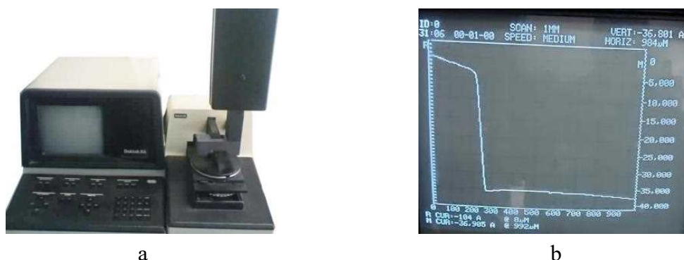
Fig. 1. The Sloan Dektak IIA profilometer (a) and the etching depth of the Ge sample surface at the interface of the photoresist-protected area and the surface etched for 42 min (b).
