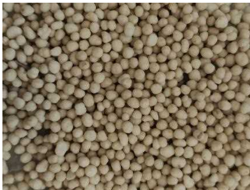
Fig. 5. Photo - view of coated NCaS fertilizer granules.
