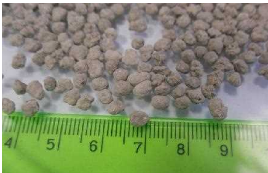
Fig.1. Photograph of the adduct obtained in the semi-technical plant test in 2011.
